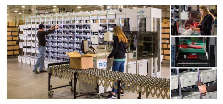
Sure Sort is a highly scalable, configurable and cost-effective small-item robotic sorting system that delivers a wide variety of parcels and individual items in a single pass. Its smart automation is based on proven iBOT® delivery technology
